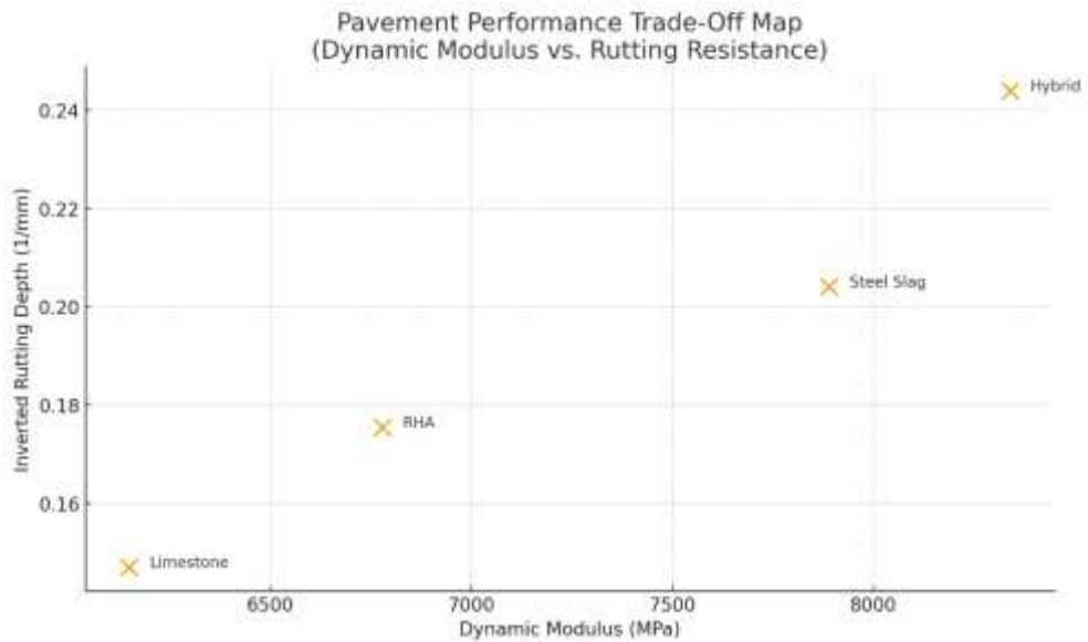
Figure 3. Dynamic modulus vs. rutting resistance for asphalt mixtures — hybrid filler (slag + RHA) occupies the top-right corner with the highest stiffness and lowest rutting depth, confirming synergistic performance.
